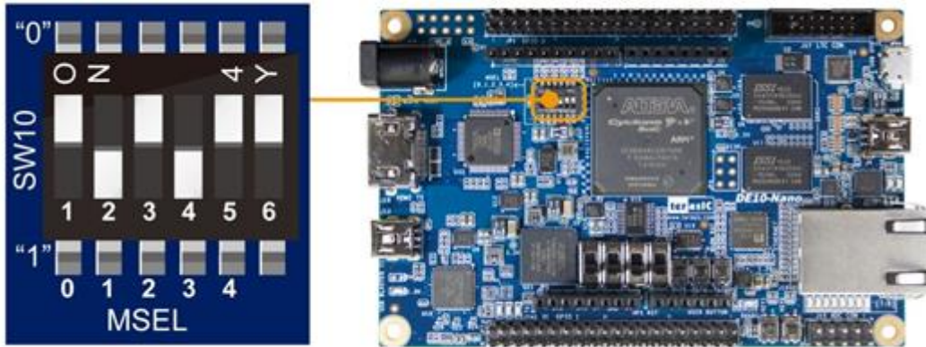
Figure 7-3 Set MSEL[4:0] to "01010" for ARM Version Mode
