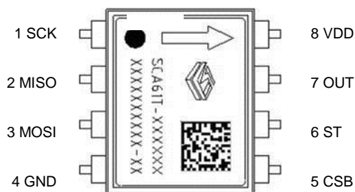
Figure 3. SCA61T electrical connection
